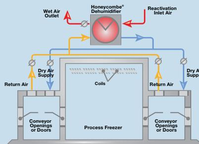
Fig. 2 Air System with Vestibule
