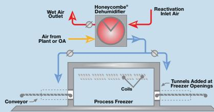
Fig. 1 Make-up Air System with Tunnels
